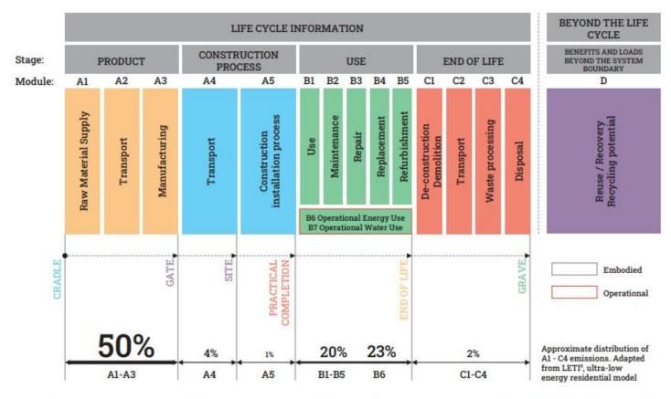
Fonte: BS EN 159783 Life cycle stages using example data across all building elements (estratto da "How to calculate embodied carbon" - The Institution of Structural Engineers)
